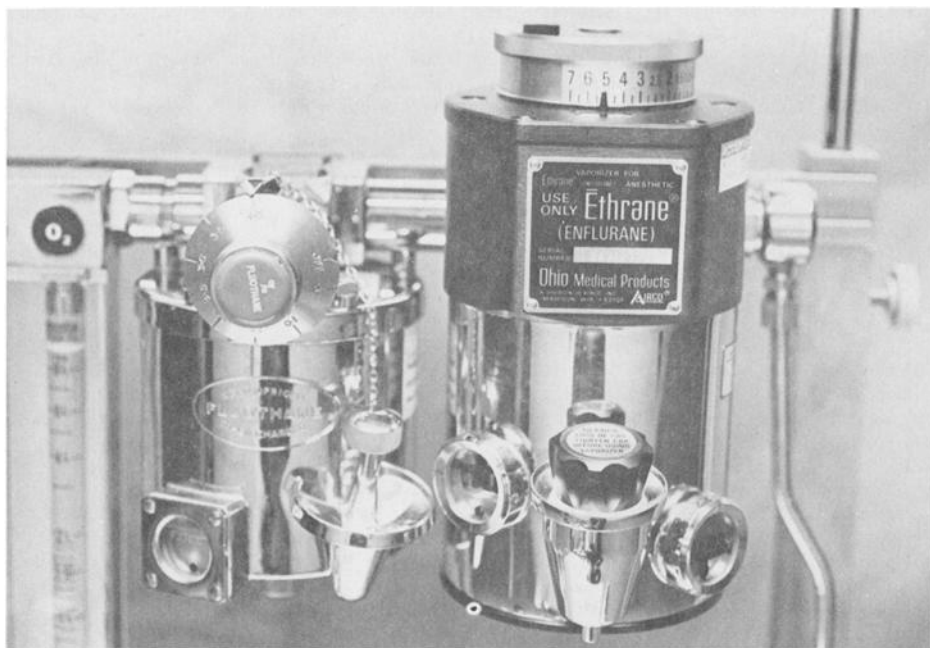
FIG. 2—Close-up of the vaporizers shown in Fig. 1. The close-up illustrates the degree of visual attention the operator must expend to accurately assess the control valve settings.
